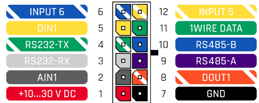
Figure 2 FMB125 2x6 socket pinout
