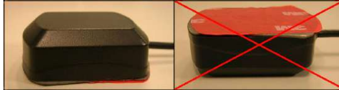
Figure 86 FMB122 and FMB125 GNSS antenna correct and wrong position
